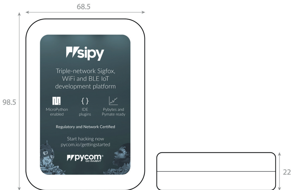
Figure 10 – Mechanical drawing of packaging – Units: mm
