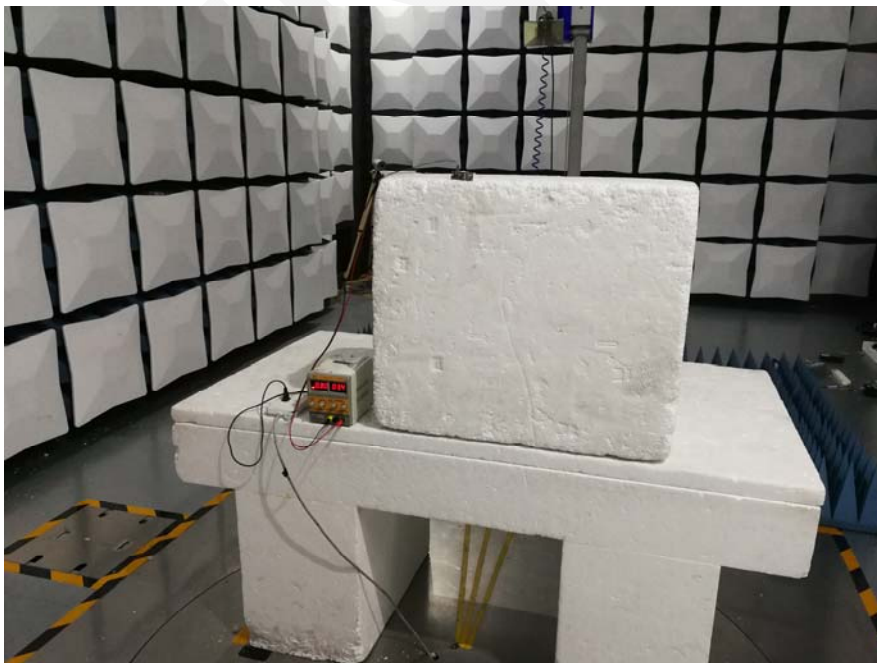
Radiated Spurious Emissions Test View (Above 1GHz)
